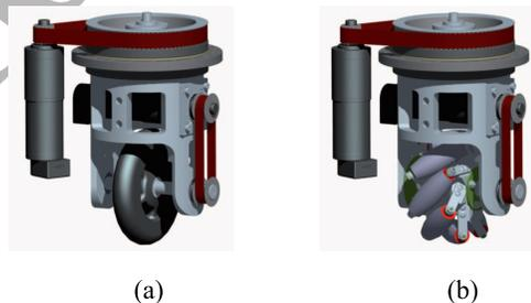
Fig. 7. Drive unit with standard and omni-directional wheel
