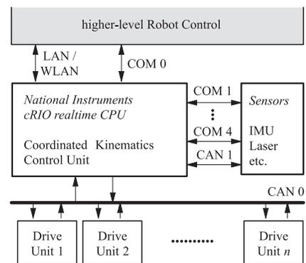
Fig. 11. Control architecture
