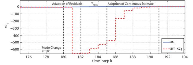
(a) Continuous state deviation due to the mode identification delay for a mode change  $q_2 \rightarrow q_4$
