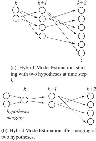
Fig. 6. Comparison of the number of mode hypotheses generated by the hME (a) with and (b) without hypotheses merging.
