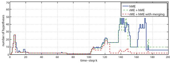
Fig. 8. Comparison of the number of considered hypotheses at each time-step  $k$  for the standard hME algorithm and the new ARR focused approach (rME und hME).
