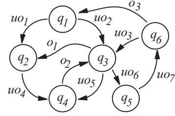
Fig. 1. Discrete automaton with six operational modes.
