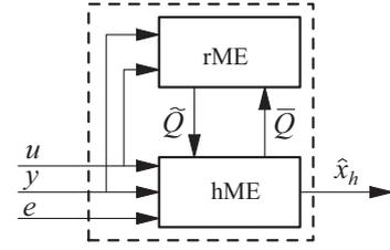
Fig. 3. Hybrid estimation architecture.
